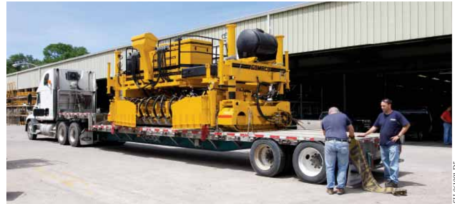
The GP-2400 was designed for transportability between job sites.
