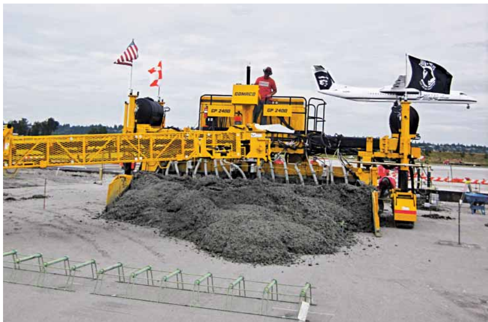
The GP-2400's pedestal console is hinged, allowing it to shift forward for paving and retract back in for minimum shipping requirements.
