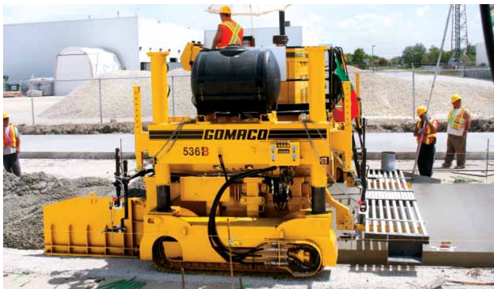
A GP-2400, two-track, paves a 16.4 foot (5 m) wide, eight inch (203 mm) thick slab for a parking lot.
